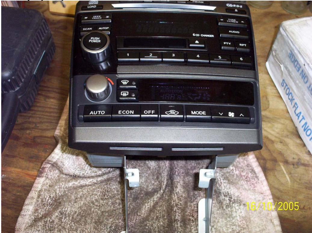
Stereo and climate control units removed from vehicle
